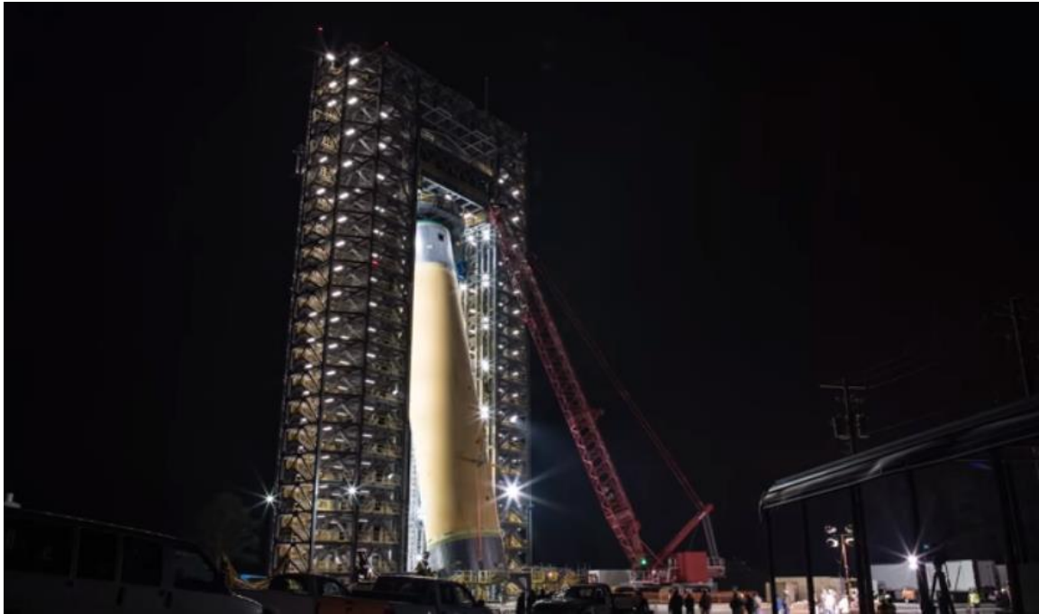
Lift the SLS Liquid Hydrogen Tank Test Article in Test Stand
