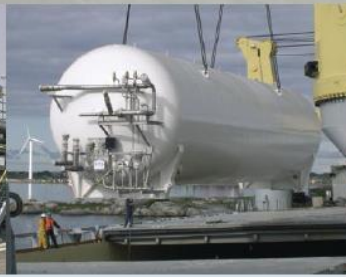
300 m 3 storage tank for LH_2
