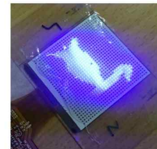
Figure 6. A backplane of AM mini-LED with LEDs.
