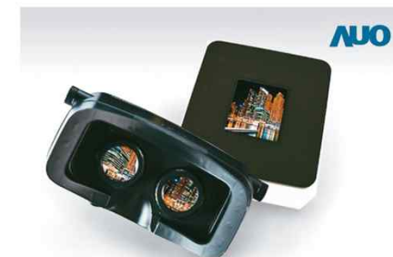
Figure 7. A 1000PPI VR LCD module with AM mini-LED embedded.
