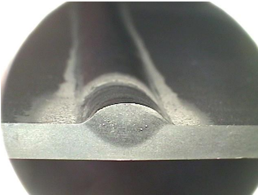
ac-TIG welding (with filler metal)
